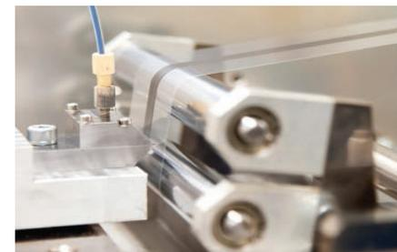
Microgravure/slot die coating machine in the Birck Nanotechnology Center.
